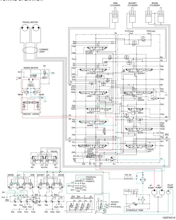
When the left control lever is pushed left or right, the swing spool in the main control valve is moved to the left or right swing position by the pilot oil pressure (Pc2, Pd2) from the remote control valve.
