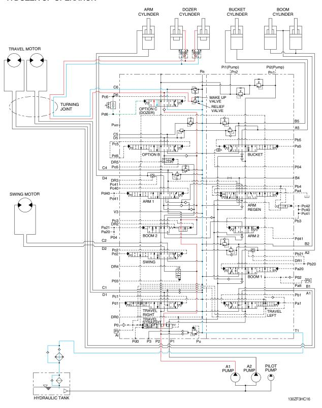
When the dozer control lever is pulled back, the dozer spool in the main control valve is moved to the dozer up position by the pilot oil pressure (Pd6) from the remote control valve.
