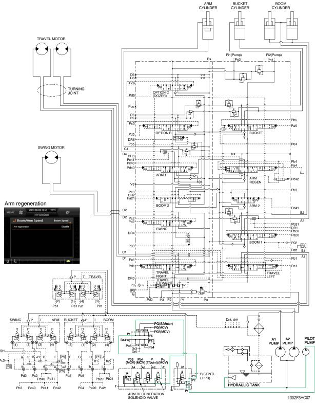
When the arm regeneration is selected to disable on the cluster, the arm regeneration solenoid valve is activated. The pilot oil from pilot pump flow into **Pb4** port in main control valve through solenoid valve and the arm regeneration spool is shifted to left.
