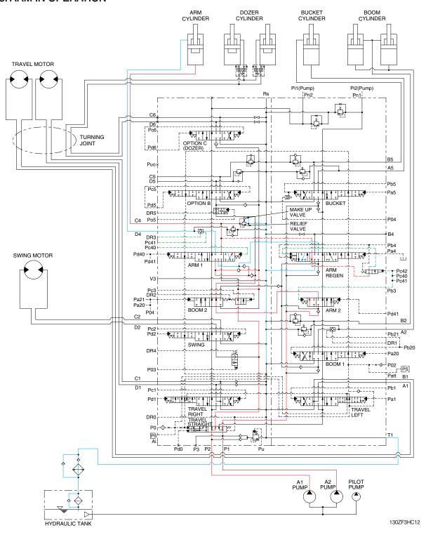
When the left control lever is pulled back, the arm spools in the main control valve are moved to the arm in position by the pilot oil pressure (Pc40, Pb3) from the remote control valve.
