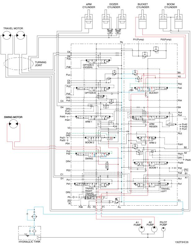
When the swing and bucket functions are operated simultaneously, the swing spool and bucket spool in the main control valve are moved to the functional position by the pilot oil pressure (Pc2, Pd2, Pa5, Pb5) from the remote control valve.
