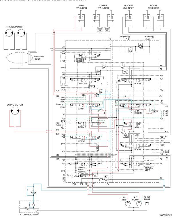
When the swing and arm functions are operated simultaneously, the swing spool and arm spools in the main control valve are moved to the functional position by the pilot oil pressure (Pc2, Pd2, Pc40, Pb3, Pd40, Pd41) from the remote control valve.
