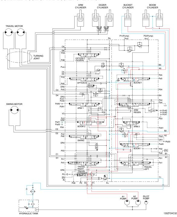
When the boom up and bucket functions are operated simultaneously, each spool in the main control valve is moved to the functional position by the pilot oil pressure (Pa20, Pa21, Pa5) from the remote control valve.
