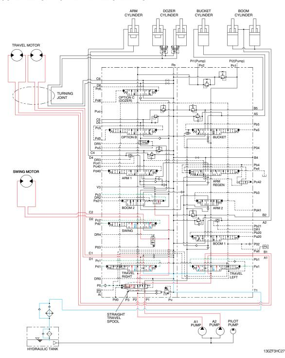
When the swing and travel functions are operated simultaneously, the swing spool and travel spools in the main control valve are moved to the functional position by the pilot oil pressure (Pc2, Pd2, Pa1, Pb1, Pc1, Pd1) from the remote control valve and straight travel spool is pushed to the right by the pilot oil pressure from the pilot pump.
