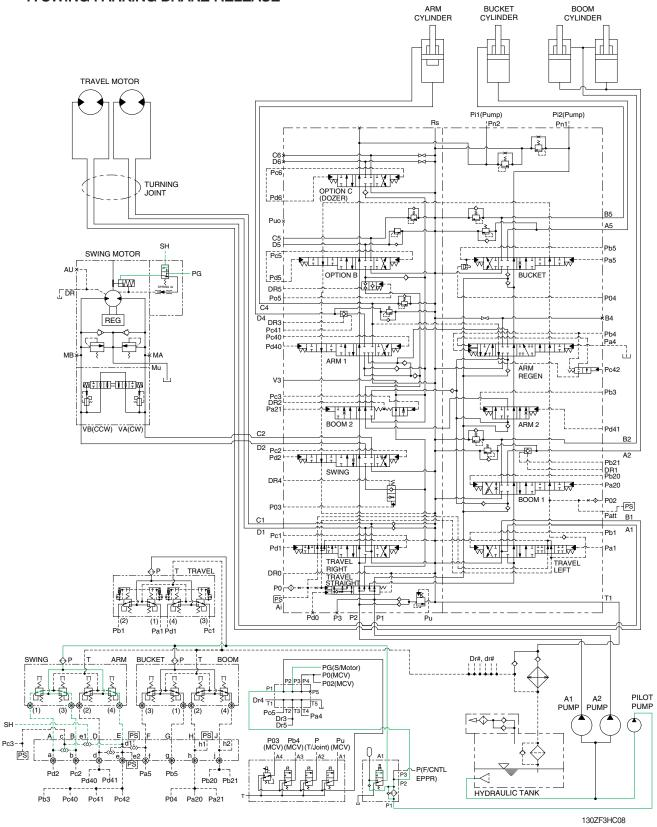
When any lever of the swing, arm in, boom up or travel is tilted, the swing brake solenoid valve is shifted to the downward by the MCU that senses the pilot pressure of the RCV control lever.
