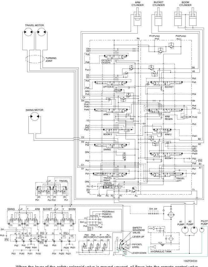
When the lever of the safety solenoid valve is moved upward, oil flows into the remote control valve through the line filter, safety solenoid valve and cross assy.
